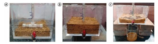
Figure 8. Typical experiment to simulate water leakage from a pipe. a, Mould filled with soil and underwater pipe. b, Soil filled with leakage from pipe. c, Soil layer after pipe leakage and the soil fines are lost.
