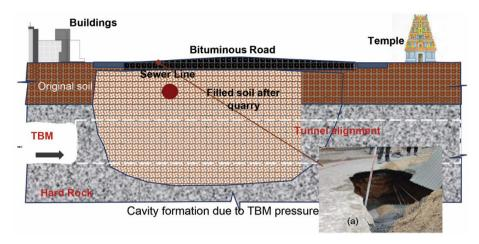
Figure 6. Blow-out cavity formation due to underground tunnelling work in a city.
