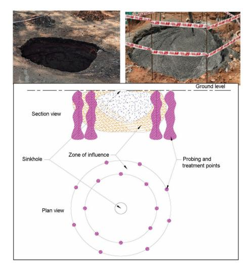
Figure 9. Treatment of urban cavity close to a metro project.
