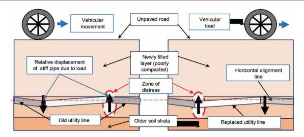
Figure 7. Breakage of utility pipes (laid in poorly compacted backfill) due to uneven settlement of surrounding media caused by uneven compaction from vehicular load.
