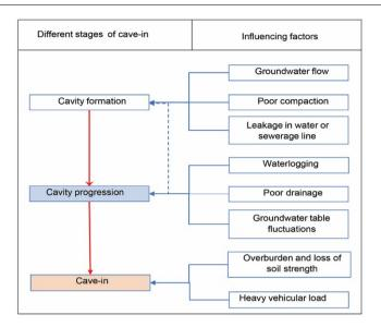
Figure 3. Factors affecting different stages of cavity/sinkhole formation.
