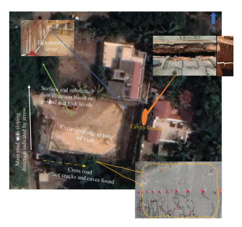
Figure 4. Typical surface cracks and cavity formation due to excavation and dewatering.
