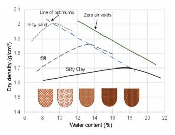
Figure 5. Typical compaction plot of different soil types and the effect of water content.
